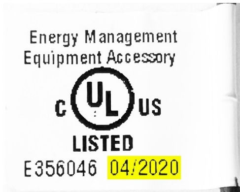
Figure 6. Old EFC UL label date code “04/2020” MM/YYYY (yellow highlight)
