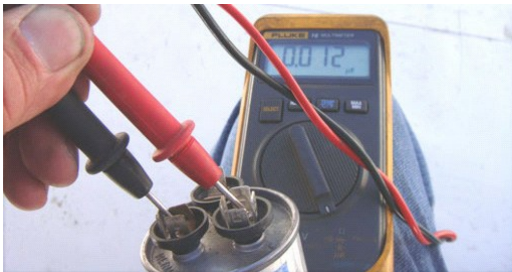
Figure 4. Checking 50 \mu F capacitor but only measuring 0.012 \mu F indicating failure
