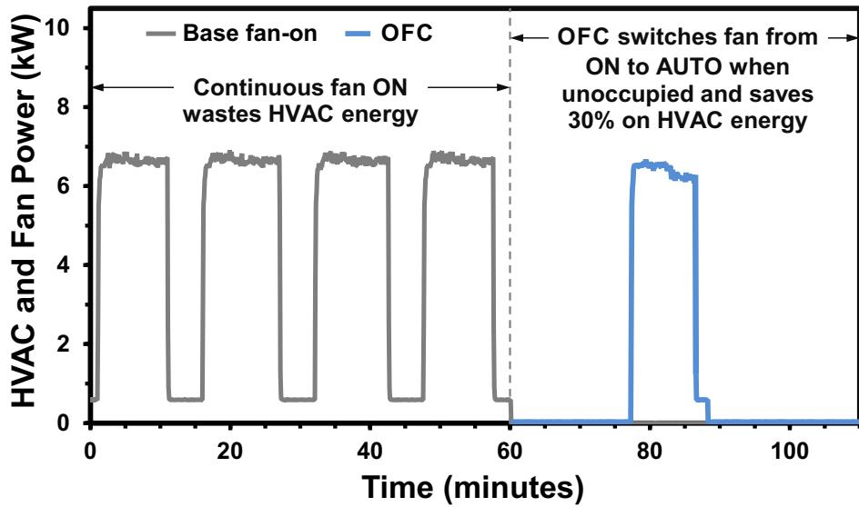
**OFC** variable fan-off delays save 8 to 15% on heating and cooling based on Intertek laboratory tests and cooling fan-off delay prevents biofilm on evaporator coils.
