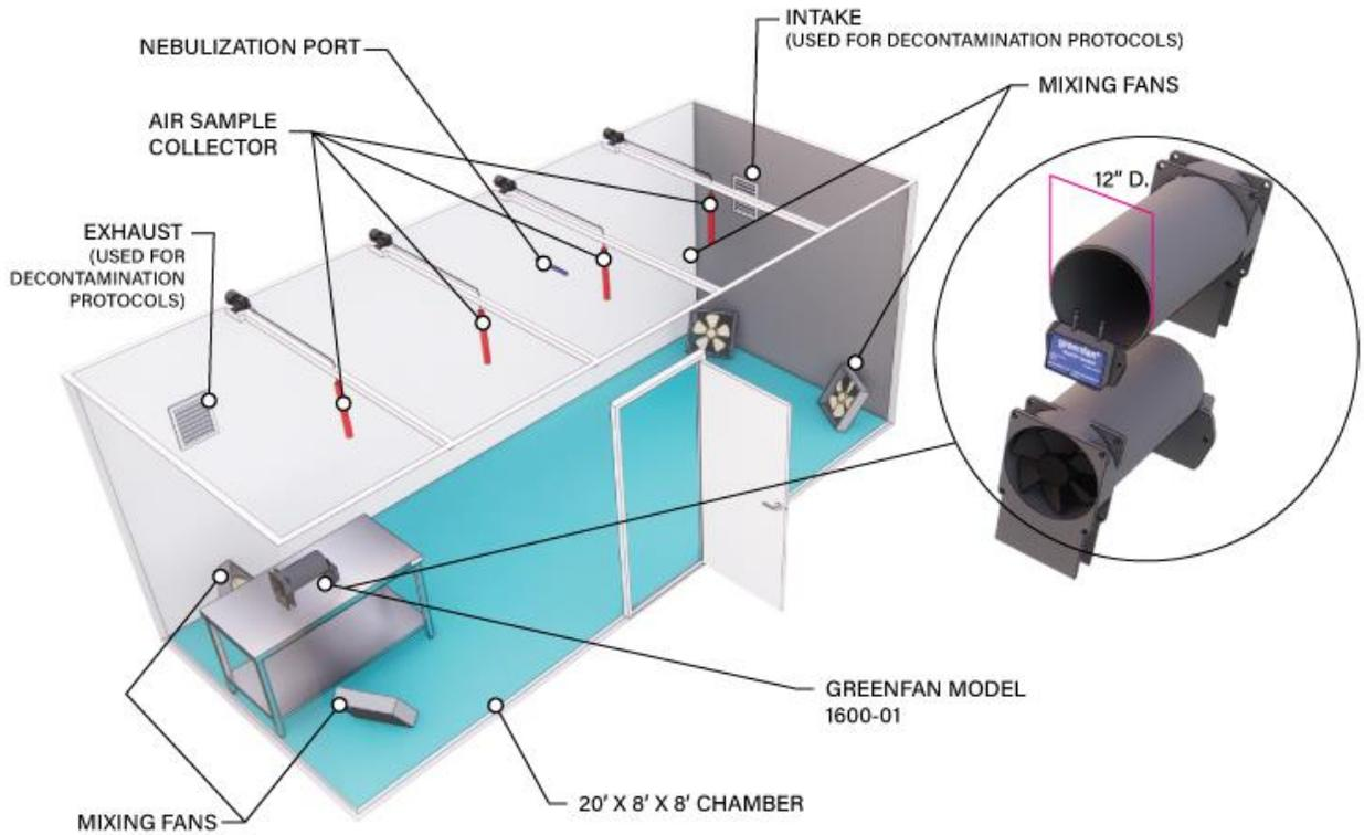
Figure 4. Testing layout for control and experimental trials. Testing chambers exhaust and intake are not used during active virus testing outside of the decontamination function.
