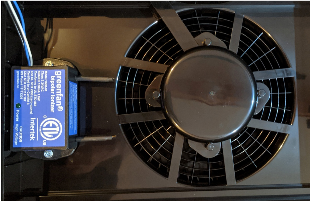
Figure 10. greenfan® bipolar ionizer installation at fan inlet of an air purifier
